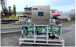
Earlier in the summer, the team at Harmony Desalting visited Singapore to deliver their first seawater desalting pilot, *Searay*. Due to the high salinity of seawater (35,000 ppm) this system was built to operate at higher pressures: up to 83 bar (1200 psi). By operating at variable salinities and pressures, *Searay* can reduce energy demand by 30% or more compared to standard RO processes.
