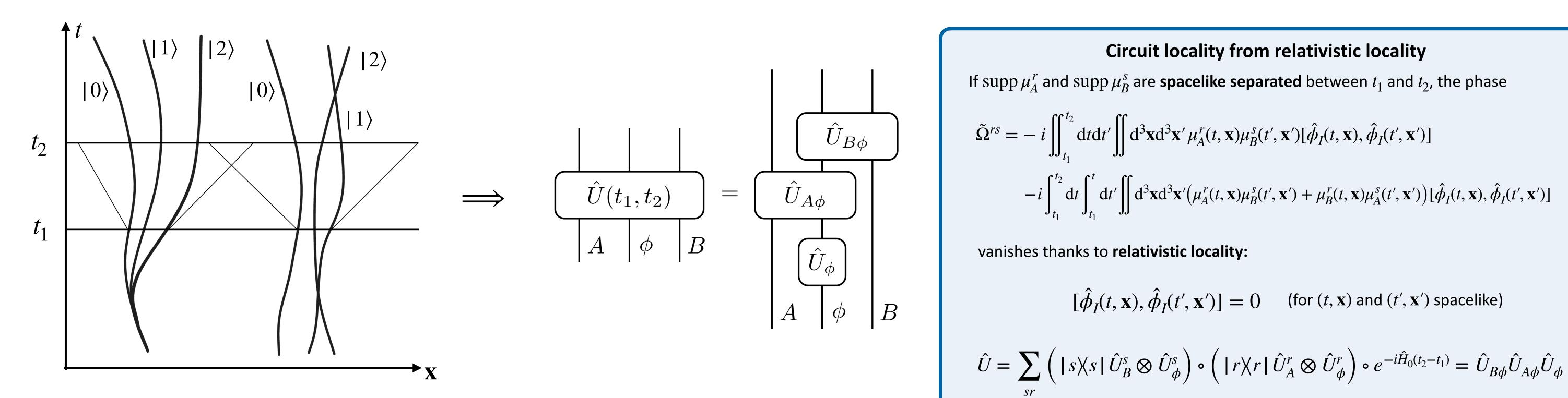
quantum-controlled superposition of localised states + spacelike separation  $\implies$  circuit-local evolution
